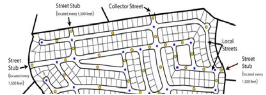
Figure 22 –Example of a diagram illustrating the Connectivity Index.
